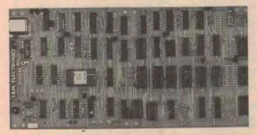
Two versions are available: (1) EMI-3A: 64x16. Upgrading to 80x24 is possible by the addition of extra components.
