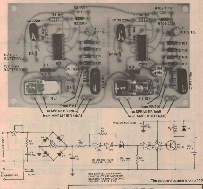
loudspeaker protector experimentally rather than just setting it to the rated power handling of your loudspeakers. Your ears are the best indication that the system is being strained. Set the loudspeaker protector so that it trips just below that volume where distortion starts to occur.
