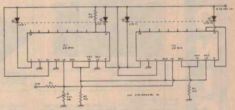
Figure 8. Dot mode voltmeter with 20 LEDs. Full scale is 2.4 V when Rx is zero.
