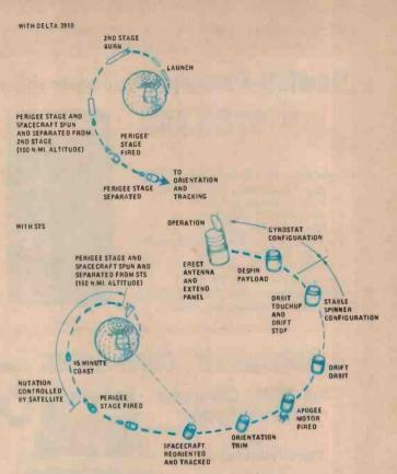
Figure 3: It is hoped to launch the SBS craft using the Shuttle, but as the Shuttle may not be available early enough for the first launchings, provision has been made for a rocket launch. In both cases the satellite will take up a geosynchronous orbit.
