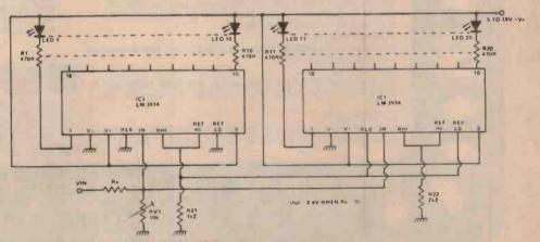
Figure 9. Bar mode voltmeter version of above.
