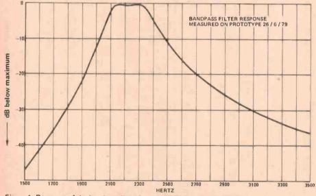
Figure 1: Response of the bandpass filter for the RTTY decoder (ETI-730).
