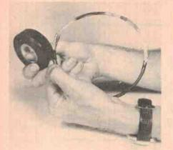
1: Having wound the coil as described, wrap it with two layers of insulation tape.
