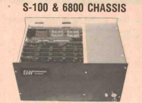
11 slot backplane, fully card guided. 15 amp power supply, fan, key switch, bench mount, rack mount, annodised aluminium. 5 edge connectors stan-dard. S-100 Bench Kit \$345. S-100 Rack Kit \$306. 6800 Bench Kit \$370. 6800 Rack Kit \$330. Assembled prices add \$100.
