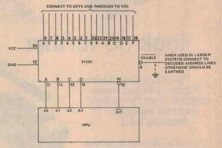
plexers, 16 lines each and using more address lines to enable each multiplexer one at a time (i.e. short form ASCII-6 bits can be encoded by four multiplexers, four lines address all multiplexers and the other two lines select only out of four multiplexers to be enabled).
