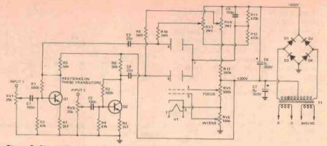
Figure 6: Circuit dlagram of the tuning oscilloscope. V1 is a 913 25 mm (1") CRT obtained from surplus sources. Many an amateur junk box will contain one – ask around. Virtually any tube up to 75 mm diameter will suffice.
