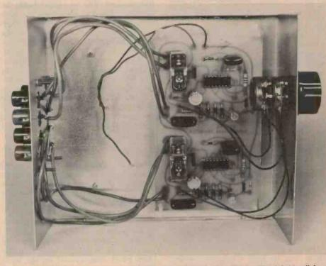
Internal view of the speaker protector. We mounted the unit in a 'Deluxe Metal Cabinet'' from Dick Smith measuring 184 x 160 x 70 mm, but you can choose any similar size cabinet to suit your equipment or even mount single units in your loudspeaker enclosures with preset controls.
