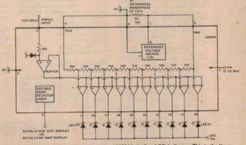
Figure 2, Equivalent internal circuit of the LM3914 dot/bar LED indicator. This is the linear indicator chip in a series of three – the '15 is a log type, the '16 a VU type.
