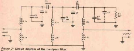
The inductors, L1, L2, L3 are 88 mH toroids or pot cores (see text). Refer to text for C2, C5 and C8.
